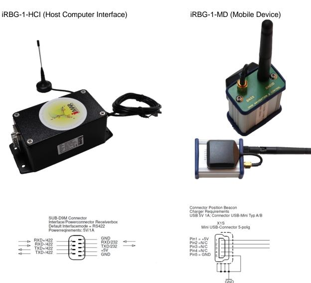
The Mobile Device provides an USB interface for battery charging (5 V, 1 A) and configuration.
