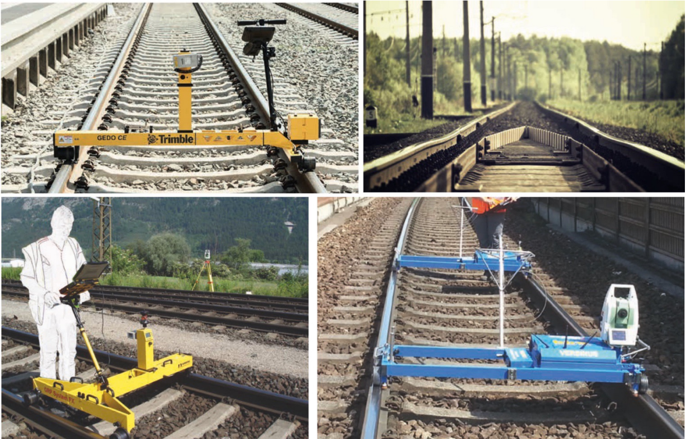
Figure 1: From upper left, counterclockwise: examples of hand operated manual measurement/surveying of track parameters, Upper right: plastically deformed rail tracks [2]
