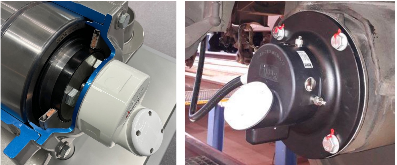
Figure 13: iMAR Navigation GmbH iRAD prototype, with axle generator (left), mounted on the Mewa12 axle (right)
