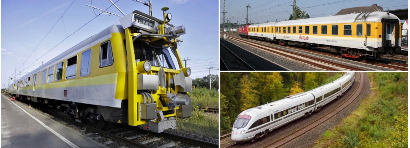
Figure 2: Measurement Trains of Deutsche Bahn AG (DB): from left clockwise, LIMEZ III train, RAILLab, Advanced TrainLab - all equipped with Inertial Sensing from iMAR Navigation GmbH
