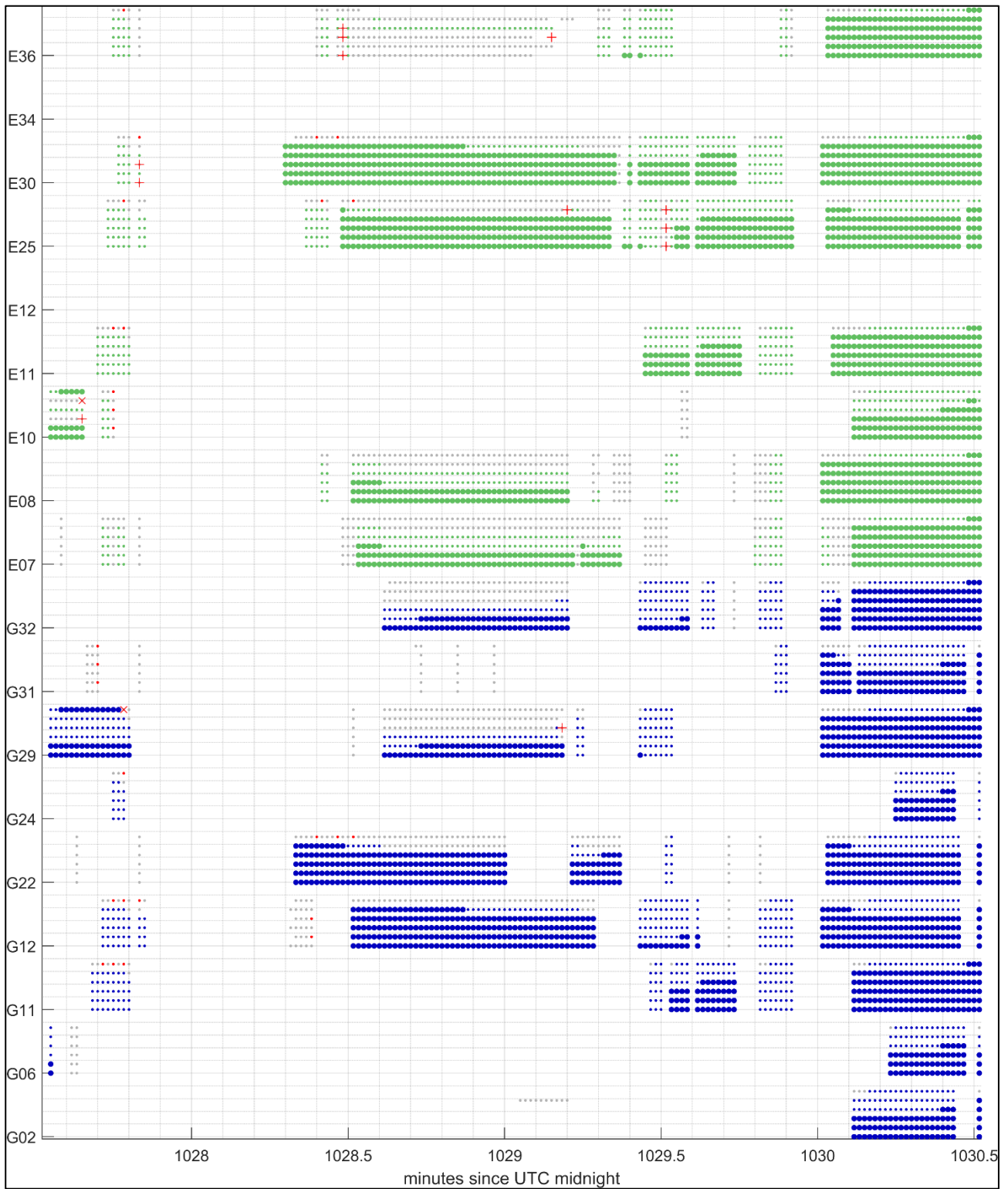
Figure 7. Development of ambiguity fixes over 6 EKF-passes for tightly coupling with a navigation grade IMU (iMAR RQT); section 4 (urban canyon) with very challenging GNSS conditions. Data rate is 1 Hz. Grey dots: float phase observation; colored thin dots: wide-lane fixed phase observation; colored thick dots: fully fixed phase observation; red '+': Outlier.
