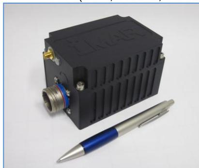
three MEMS accelerometers and an integrated powerful micro-processor with >20 bit sensor data digitalisation included to provide digital data transmission (CAN, RS232, RS422) and extended internal error modelling with high bandwidth. As an option an internal GPS or/and external magnetometer can be provided as well as a wheel sensor to achieve higher performance also in
