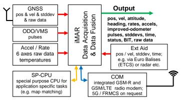
**iRailLoc-C** is, as all iNAT systems, delivered with the MS-Windows (or LINUX or MacOS alternatively) based configuration software <u>iXCOM-</u> <u>CMD</u>. This software allows to configure the output interfaces. Furthermore, all output data can be displayed and stored online on the user's notebook, tablet or process computer. It also allows powerful playback capabilities and provides data export in many formats (csv, xml, GoogleEarth<sup>™</sup> etc.). Python and MatLab interface available.
