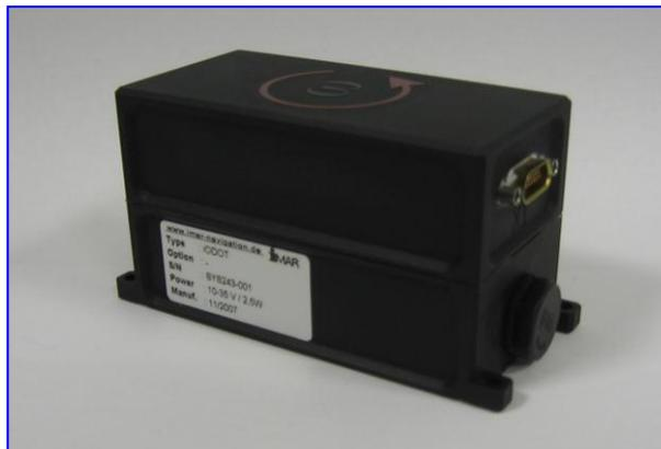
The iODOT comes in an ruggedized aluminum housing and contains the fiber optical sensing unit with fiber coil followed by high sophisticated analog and digital signal processing. The digital compensated output has a linearity error < 1 % (inside +/- 100
