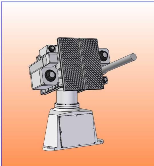
Mounting the camera on a stabilized gimballed platform achieves the dynamic separation of the
