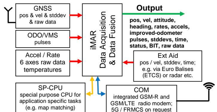
**iRailLoc-C** is, as all iNAT systems, delivered with the MS-Windows (or LINUX or MacOS alternatively) based configuration software **iXCOM-CMD**. This software allows to configure the output interfaces. Furthermore, all output data can be displayed and stored online on the user's notebook, tablet or process computer. It also allows powerful playback capabilities and provides data export in many formats (csv, xml, GoogleEarth™ etc.). Python and MatLab interface available.
