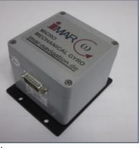
speed digitization and microprocessor ิล based signal processing the iMGYR-SN provides an output signal being proportional to angular velocity. The integrated micro-processor reduces the nonlinearity to much less than 0.2% f.s and compensates the bias on the digital and analog output
