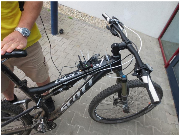
Figure 1: Mountain Bike with installed reference measurement system i \mu VRU
